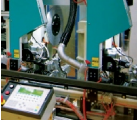
Ultrasonic torsional welding system with 500 W output power, suitable for integration into automatic production lines
